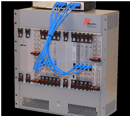
FLEX digital control electronics can be located in a climate controlled cabinet in the utility box or inside the vehicle.
