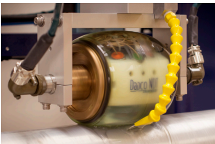
Nordco 9-channel inspection wheel probe
