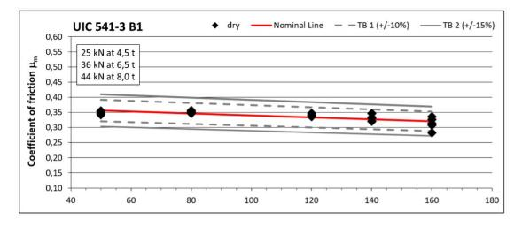
Typical friction coefficients for axle-mounted discs according to UIC program S1 (200 km/h) and EN15328. The tested pad was the FP 94.
