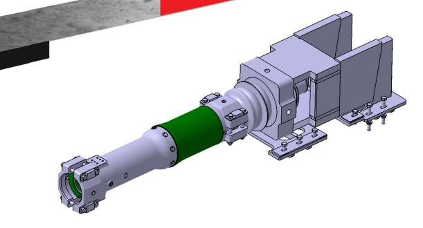
Description : The semipermanent couplers are provided between the coaches and at the loco and coach connection. A muff coupling is used to join two semipermanent coupler halves. The couplers are physically validated for high compressive load capacity of 2000 kN, tensile load capacity of 1000 kN and bending load capacity of 300 kN.
