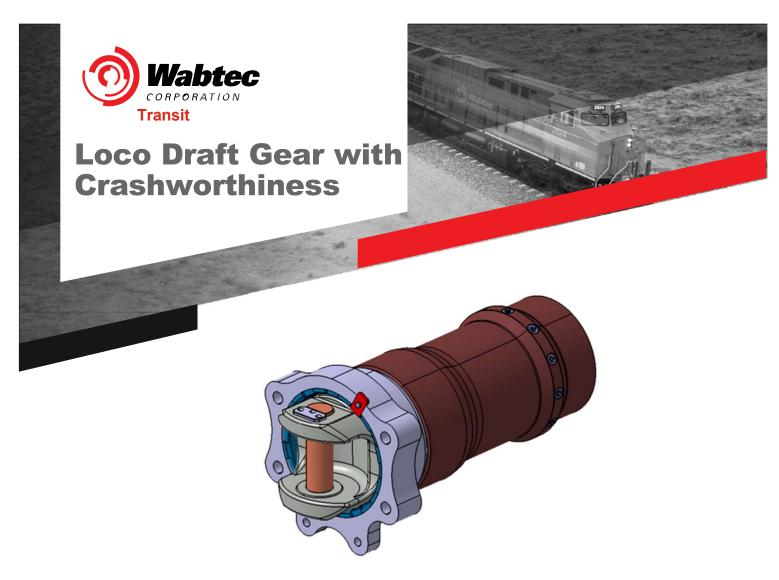
**Description:** Crashworthiness is ability to mitigate the consequences of a collision in a controlled manner and reduce the risk of injury to the occupants. Car-body flange act as assembly interface (via bolting) with car-body plate. Deformation tube is welded to car-body flange.
