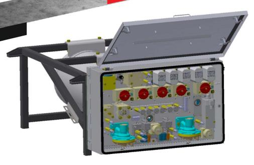
**Description :** The brake module supplies pressure to Brake Cylinder line( BC) through Relay valve, piloted by an electro-pneumatic circuit comprised of solenoid valves and pressure transducers operated in closed loop by microprocessor-controlled Electronics.
